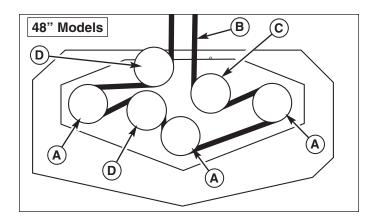
Figure 14. Mower PTO Belt Routing
